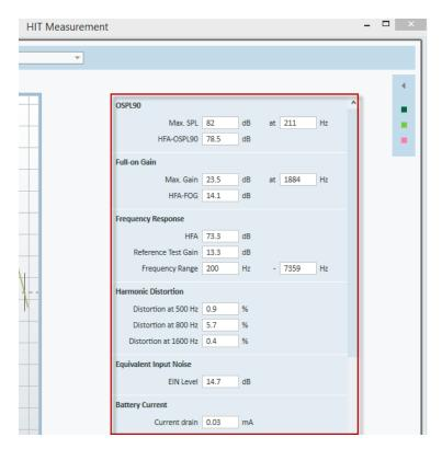
**Note:** If RTS or RTG parameters are required for a test, you will get a notification that OSPL90 has not been measured. The message can be skipped to start the measurement.
